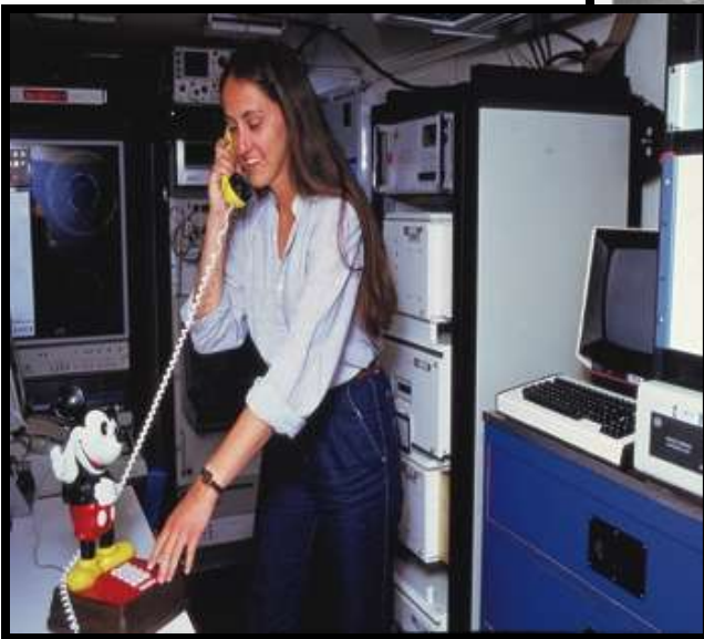
Right: Packet speech being used across internets. Speech digitization, compression, and packetizing in the equipment shown. Transmission were across the PRNet and ARPANet in tandem. SRI's Earl Craighill, head of the PR speech effort
