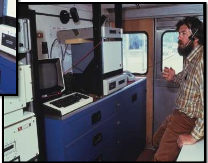
Right: Packet speech being used across internets. Speech digitization, compression, and packetizing in the equipment shown. Transmission were across the PRNet and ARPANet in tandem. SRI's Earl Craighill, head of the PR speech effort
